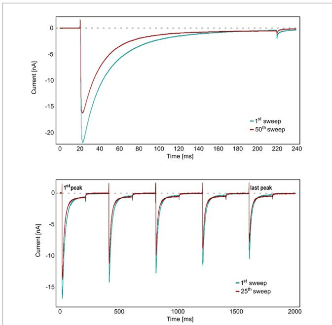
**Fig. 9:** Example current traces used for quantifying rundown. Top 1<sup>st</sup> (green) and 50<sup>th</sup> (red) depolarization in experiment block 2. Bottom: 1<sup>st</sup> (green) and 25<sup>th</sup> (red) depolarization train in experiment block 3. We quantified rundown for the first and last peak of the train.
