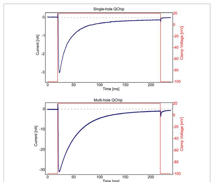
**Fig. 1:** Representative recordings of Ca<sup>2+</sup> current (blue) on a single-hole (left) and multi-hole (right) QChip following a 200 ms depolarization from -100 mV to 20 mV (red) in Ca<sub>v</sub>1.2 expressing cells.
