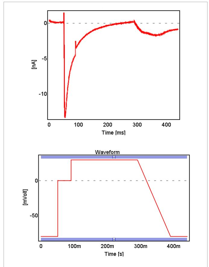
**Fig. 10:** Original recording on a multi-hole QChip of a Ca<sub>v</sub>1.2 Ca<sup>2+</sup> current (top) following a depolarization according to the CiPA protocol (bottom).
