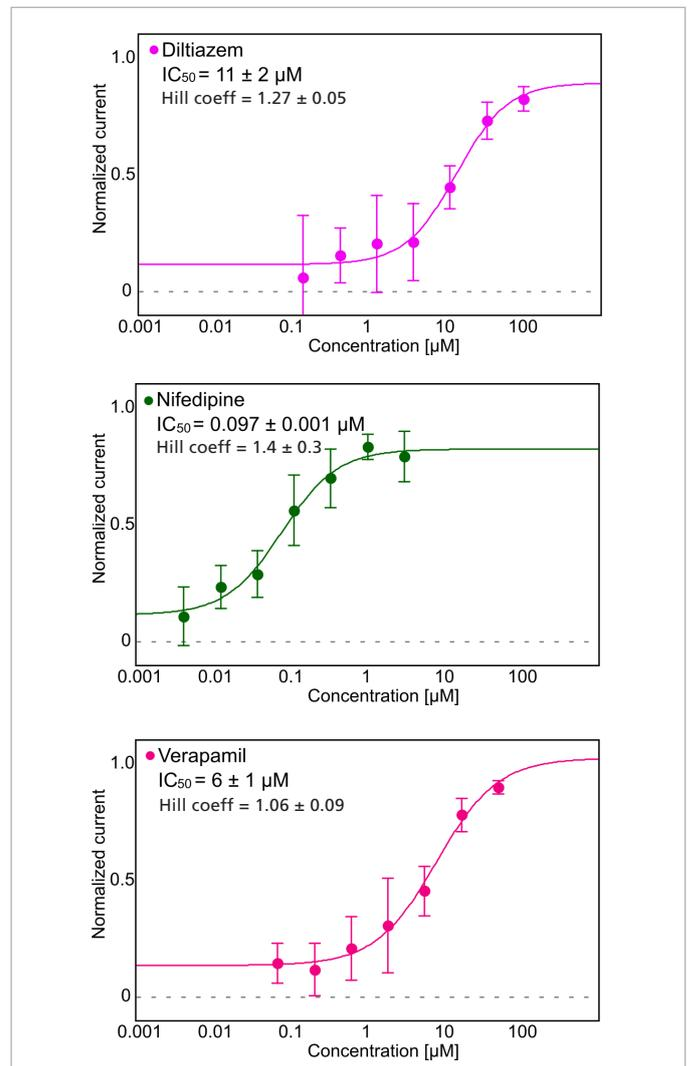
**Fig. 6:** Dose-response relationships measured using single-hole QChips for diltiazem (left), nifedipine (middle) and verapamil (right). The  $IC_{50}$  values and Hill coefficients were estimated by fitting the Hill equation to the data and the reported values are the average  $\pm$  SD of three QChips with a total of 48 experiments per compound.
