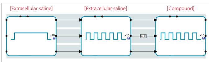
**Fig. 5:** Experiment setup in the Sophion Viewpoint software for  $Ca_v1.2$  pharmacology experiments. Voltage protocols: block 1: 10 single depolarization steps (left), block 2 and 3: 10 train depolarizations (middle and right). The compound was applied in block 3 (right).
