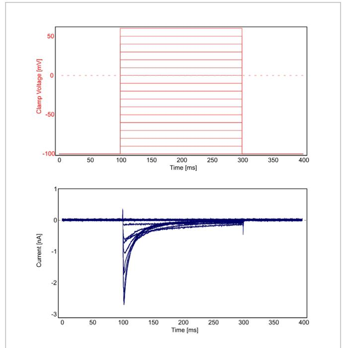
**Fig. 3:** Representative measurement of current-voltage relationship using a single-hole QChip. Top: Depolarization step protocol in  $10 \text{ mV}$  increments from  $-100 \text{ mV}$  to  $+60 \text{ mV}$ . Bottom:  $\text{Ca}^{2+}$  current response of a cell expressing  $\text{Ca}_v1.2$  channels.
