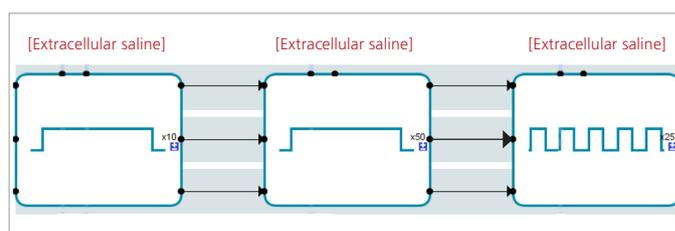
**Fig. 8:** Experiment setup for a  $Ca_v1.2$  rundown experiment in the Sophion Viewpoint software. Voltage protocols: block 1: 10 single depolarization steps (left), block 2: 50 depolarization steps (middle), and block 3: 25 train depolarizations.
