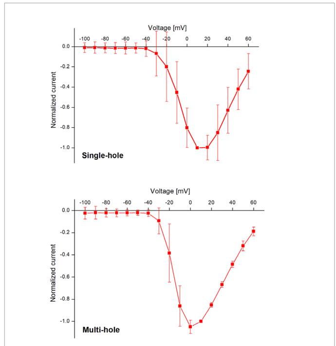
**Fig. 4:** Current-voltage plots of normalized current vs. voltage (mV) for a single-hole QChip (top) and a multi-hole QChip (bottom). The error bars are the SD.
