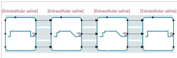
**Fig. 11:** CiPA experiment setup for a  $Ca_v1.2$  rundown measurements in the Sophion Viewpoint software. Voltage protocols: block 1 and 4: 5 single depolarization steps (15 s between sweeps), block 2: 50 CiPA depolarization steps (30 s between sweeps), block 3: 50 CiPA depolarization steps (15 s between sweeps).
