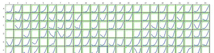
**Fig. 4:** Plate view illustrating potassium IV curves in Cor.4U cells. Only the top six rows of the QChip were loaded with Cor.4U cells.
