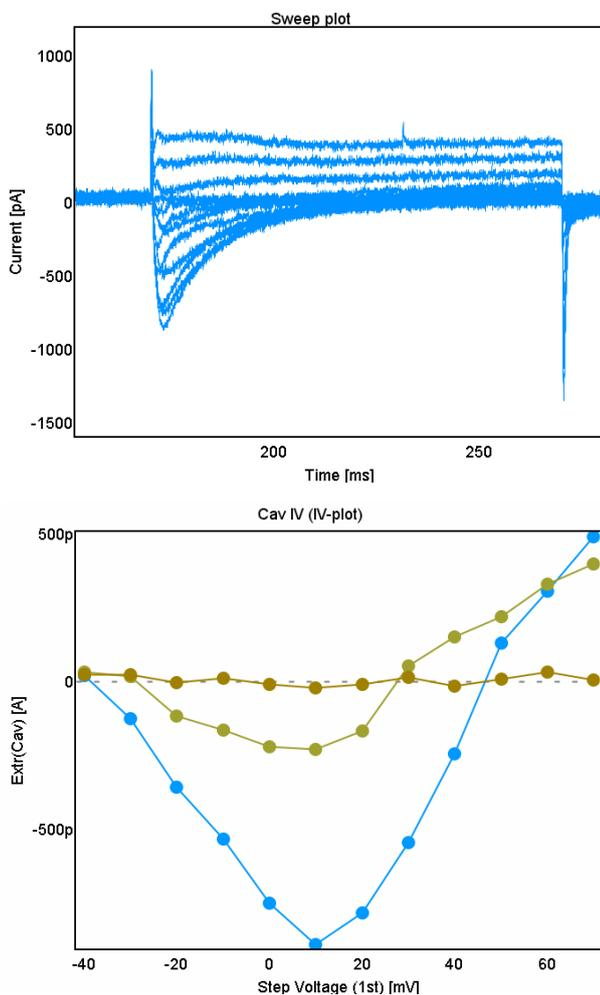
Fig. 5: Typical Ca<sub>v</sub> and K<sub>v</sub> current in a Cor.4U cell. Top panel: Current traces were evoked using a double pulse protocol with a pre-pulse to -40 mV followed by a set of voltage steps from -40 mV to +70 mV in 10 mV increments. Bottom panel: Current voltage relationship in control (blue) condition, 0.1 μM (orange) and 1 μM (red) nifedipine. The peak current measured between 2-10 ms after the voltage step was used to construct the IV curve.
