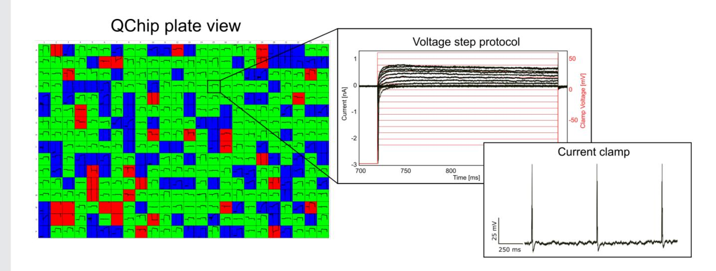
Fig. 1: High throughput measurements of hiPSC-derived motor neurons on Qube Overview of the 384-well QChip illustrating the high throughput nature of Qube measurements yielding up to 60% success rates (cell resistance > 200 M $\Omega$ ). The system allows us to perform voltage- and paced current clamp protocols within the same experiment.
